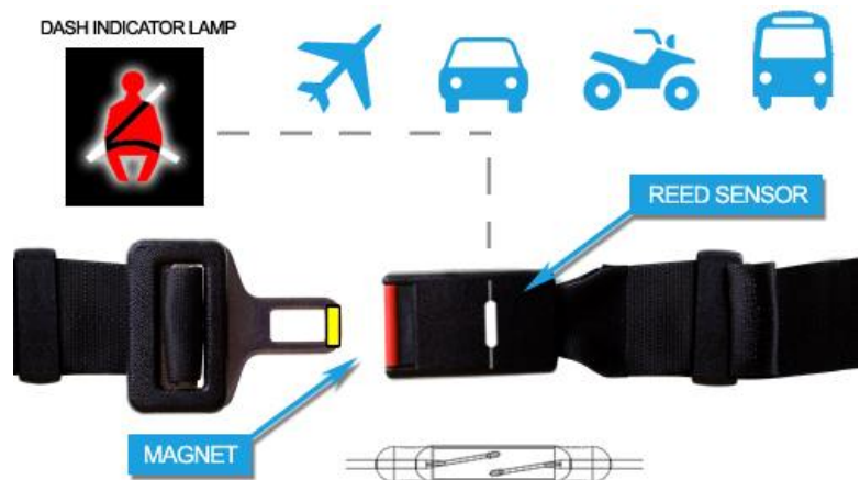
Figure 3. Shows the entire seat belt in the unbuckled position.
