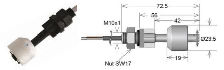
Compact single level vertical mount LSO2 Series Liquid Level Sensor used in level control, detection and monitoring. High power switch option, other cables and connectors. IP68 only up to screw in thread.
