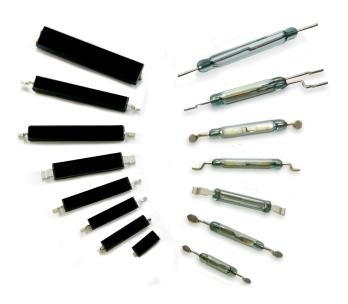
Reed switches from Standex-Meder are also robust enough to endure the conditions inside a vehicle. The switching element in their reed switch sensors is hermetically sealed, protecting the sensor from its surroundings. As a result, reed sensors can operate over a wide range of temperatures (-55°C to 155°C) and function in dirty, corrosive under-the-hood environments without any negative effects on their operating characteristics.
